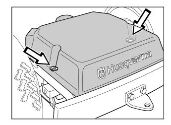
2. Check that there is oil in the transmission oil tank. Top up if necessary with engine oil SAE 10W/30 (class SF–CC).
